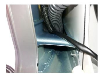
The extraction hose was then routed to an opening in the van, just above the rear towing hook.
