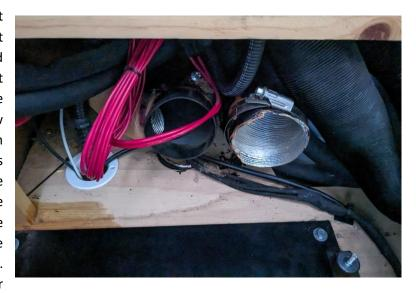
by large clamps which can be undone but I then found Murvi had put in a sneaky self-tapping screw right through the end of the pipe and into the plastic connection on the heater. I am not sure how general these are but once identified they are easily removed. The photo above shows the left hand duct missing as it disintegrated during removal. The one on the right was still in one piece but it needed replacing having grown too brittle to survive handling. The ducting is available online.
