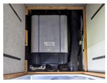
The picture above is slightly misleading as it shows two gaps in the frame on the left. I cut these after removing the heater and this made it much easier to refit the washers and nuts on this side. On first removal there were no such gaps but it was possible to get a 10mm socket onto the nuts and undo them. There are two nuts on each side which hold the heater onto rubber feet when must act to reduce noise transmission and vibration from the vehicle.
