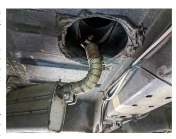
disconnected internally. A flexible pipe comes through the floor of the Murvi and then plugs into the front of the heater. It just clips into place and comes off with a pull. I accessed this area by removing one of the white vents opposite the pipe connection but I suspect you may be able to leave it in place and remove it by lifting up the front of the heater.
